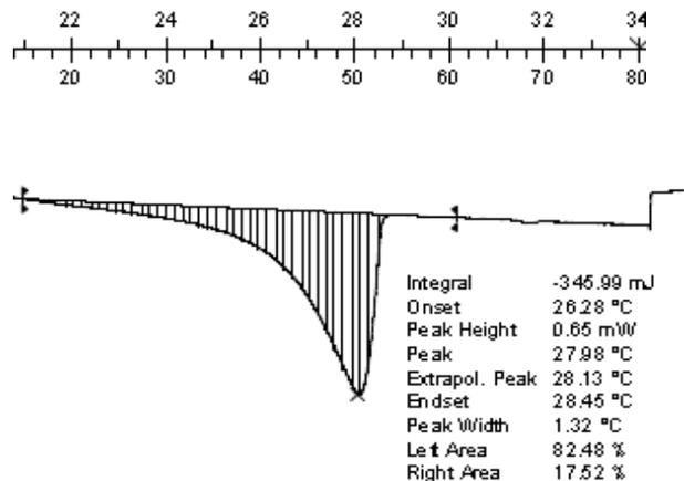
Fig 1. Enthalpy curves for microencapsulated PCM used in wallboard as measured at University of Ulster.
