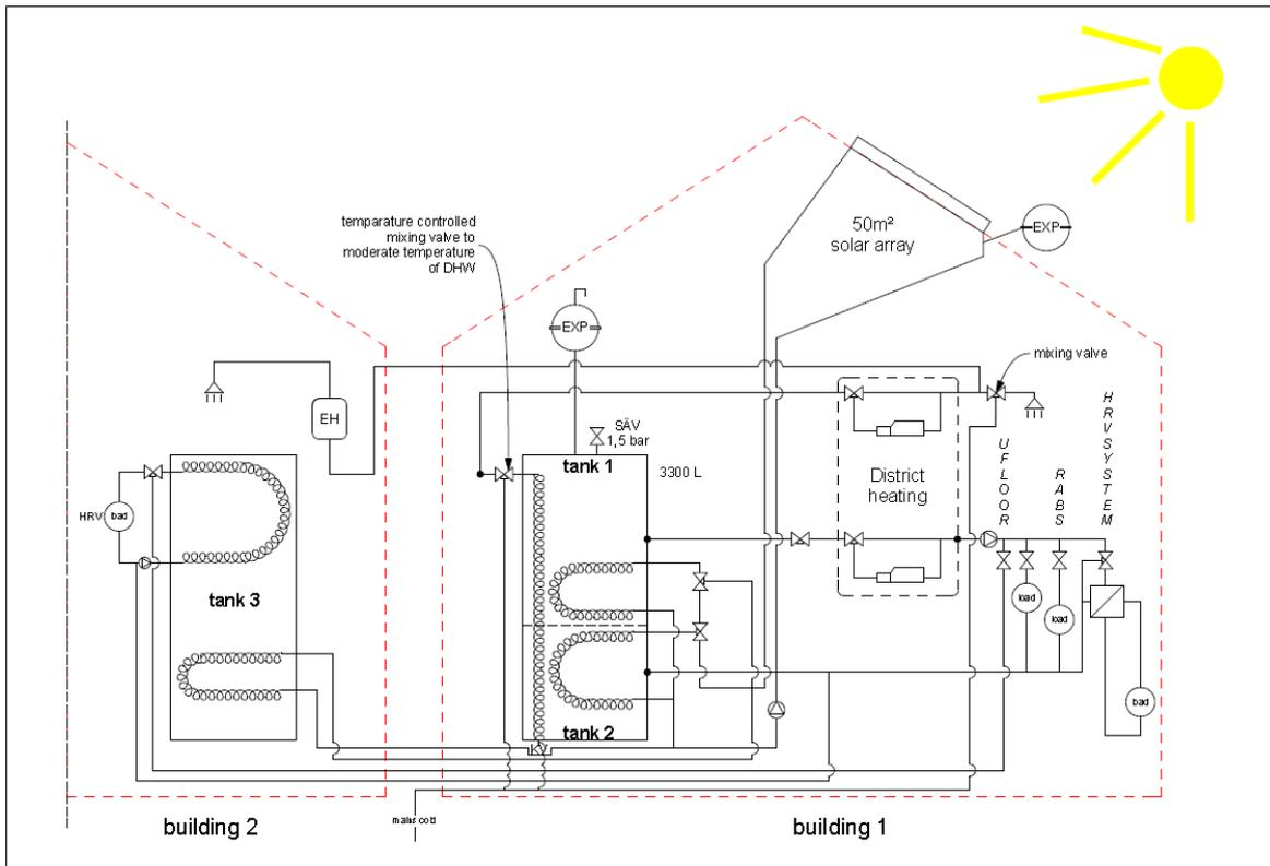
Figure 2 Schematic of heating system
